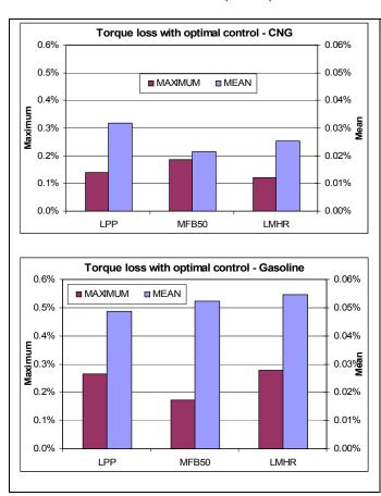
Fig. 4 Torque losses related to the indicators mean set point (Top: CNG, Bottom: Gasoline)
