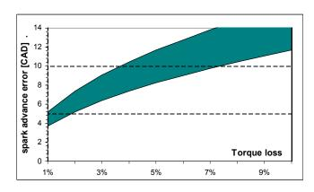
Fig. 1 Torque loss due to bad spark timing control
